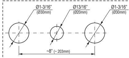
SIZE AND SPACING OF ASSEMBLY OPENINGS
